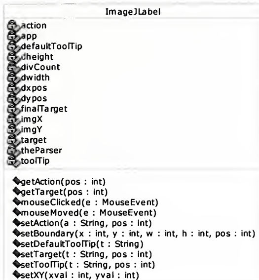
Figure 11. Class Diagram of the ImageJLabel Class
