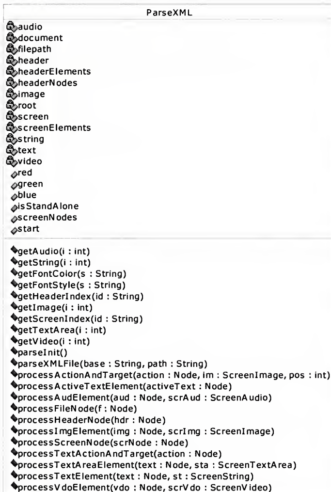
Figure 9. Class Diagram of the ParseXML Class
